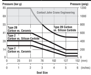
To determine the maximum pressure for the Type 2 or 2B required, multiply the maximum pressure by the multiplier factors to obtain the maximum operating pressure.
