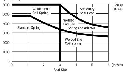
Coil spring requirements for rotating Type 1 and 1B seal heads with standard stuffing box diameter.
