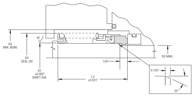
For ease of installation, the lead-in edge of shaft or sleeve should be chamfered as shown.
