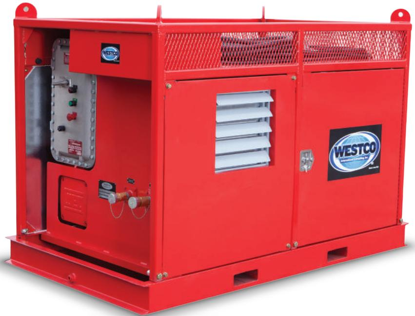
Unit is fitted with a tandem or dual stage pump. **When the Pump Control Valve is in the closed or "casing tong" position** (small 1/4" control valve located on the side of the tank), the pump automatically transitions from approx. **50 GPM at 1100 psi** to approx. **25 GPM at 2000 psi**.
