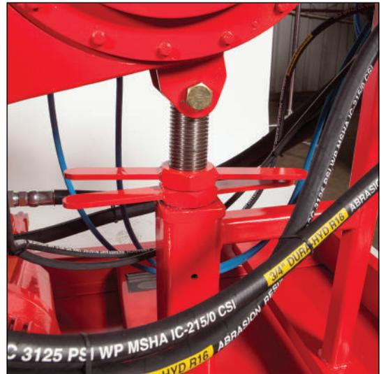
Our Bucking Unit is a portable self-contained skid mounted hydraulically powered unit that is used to make up or break out 1-5/16" up to 7" tubular connections in a horizontal position and or tool assemblies. Maximum torque of 8,000 ft-lbs.
